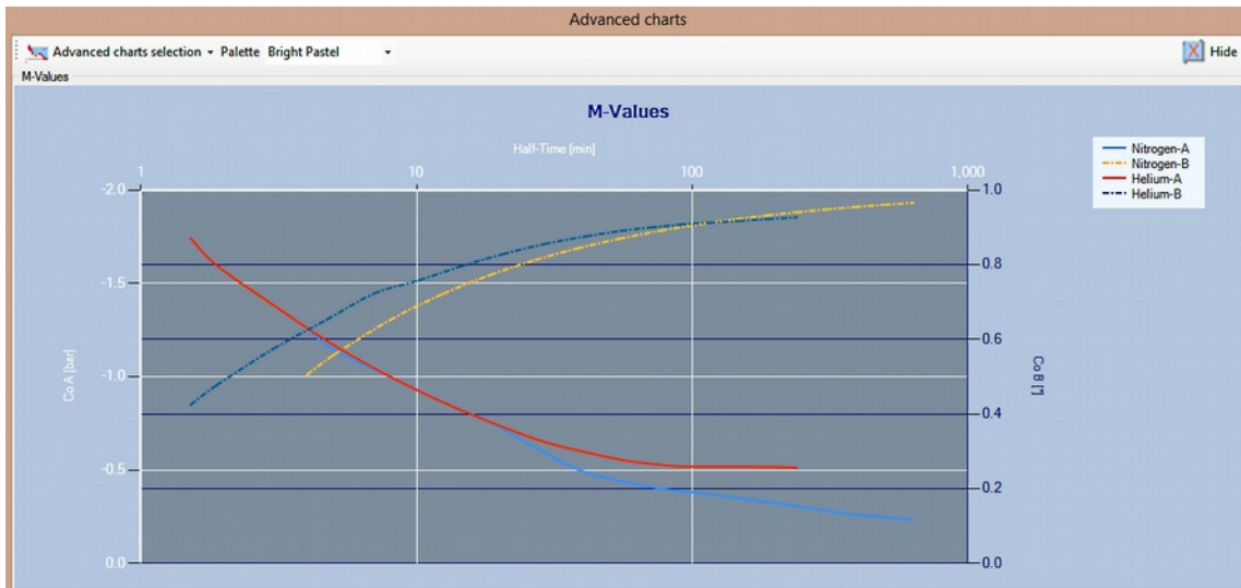
Illustration 9: Characteristic of variant of decompression algorithm
